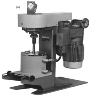
(b) Figure 10: (a) Fritsch Pulverisette P-5 Four-Station Ball Mill. (b) Schematic Depicting the Ball Motion inside the Ball Mill
