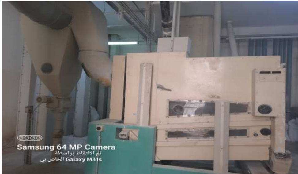
Figure 5: A Typical Cleaning Machine used in Atbara Flour Mill Factories
