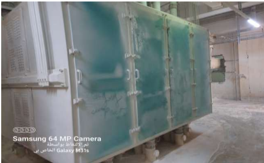
Figure 7: A Typical Main Sieve used in Atbara Flour Mill Factories
