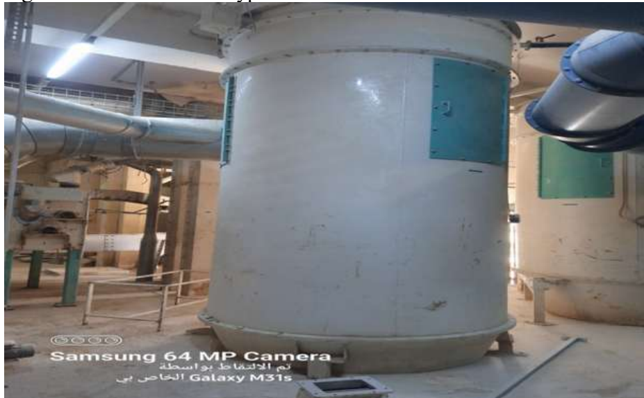
Figure 11: A Typical Flour Filter used in Atbara Flour Mill Factories
